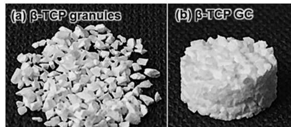
Fig. 1 Typical photo of (a) \beta -TCP granules and (b) \beta -TCP granules after mixed with an acidic calcium phosphate solution.
